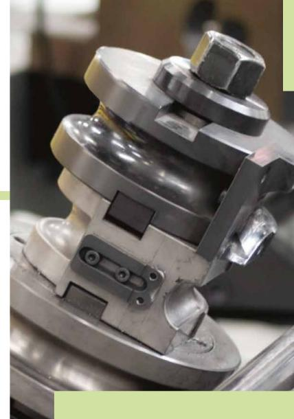
The choice fell on E-TURN40 for three reasons: fast bending tools changeover, the rotating bending head that reduce steps and the ease of use of the software.
