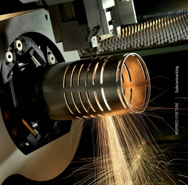
sheet-cutter with a fiber laser. Convinced of the fiber laser technology, in 2012 he added LT COM-BO equipped with a 3kW fiber laser.
