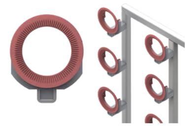
with tubular elements instead of with solid bars are more capacious for the same weight, are more resistant to deformation caused by temperature changes that characterize for example the painting jigs (they last 1000 cycles instead of the 500 of the previous fixtures), are more precise and they may contain dedicated elements that greatly simplify the loading and unloading operations made by the end customer.
