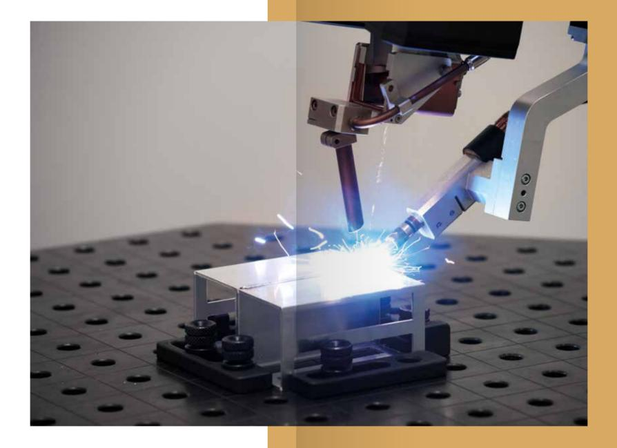
the high quality of the weld does not require subsequent rework and finishing operations of the joint thus reducing not only the overall cycle time of the assembly but also the uniformity of welds between different pieces resulting in greater control of the final quality of the welded assembly.
