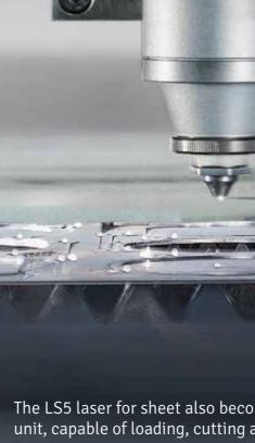
The LS5 laser for sheet also becomes a laser for pipes after attachment of the pipe module. It is actually a dual unit, capable of loading, cutting and unloading pipes, completely automatically.
